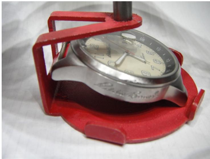
Place the watch holder assembly inside the jar and lower the watch into the water by lowering the lifting knob.
