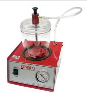
The Diablo water resistance tester functions by drawing a vacuum over the watch. The operator watches for bubbles to exit the watch which shows the location of the leak. The watch is removed from the water before the vacuum is released, preventing water from entering the case. Vacuum is much more effective at locating leaks than pressure testers. Designed, fabricated and assembled in the USA. Retail \$1250
